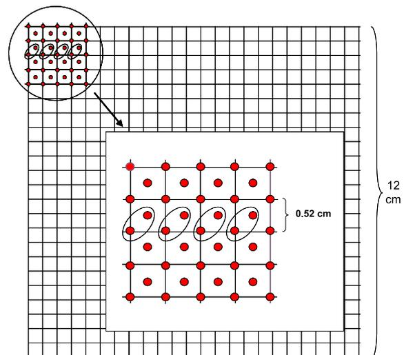
Fig. 2. Grid model for the film perforation.
