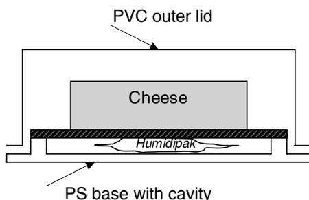
Fig. 1. Scheme of the packaging system with *Humidipak*<sup>®</sup> sachets.
