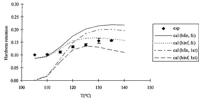
**Figure 7. Experimental hardness retention and predicted average values for a target  $F_0$  value of 5 min and static mode. Calculated profiles for first-order and fractional conversion models for finite and infinite surface heat transfer coefficients.**
