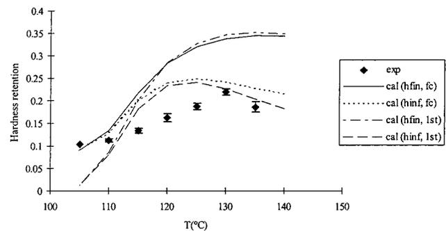
**Figure 8. Experimental hardness retention and predicted average values for a target  $F_0$  value of 3 min and 10 rpm. Calculated profiles for first-order and fractional conversion models for finite and infinite surface heat transfer coefficients.**
