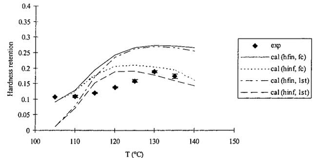
**Figure 6. Experimental hardness retention and predicted average values for a target  $F_0$  value of 3 min and static mode. Calculated profiles for first-order and fractional conversion models for finite and infinite surface heat transfer coefficients.**
